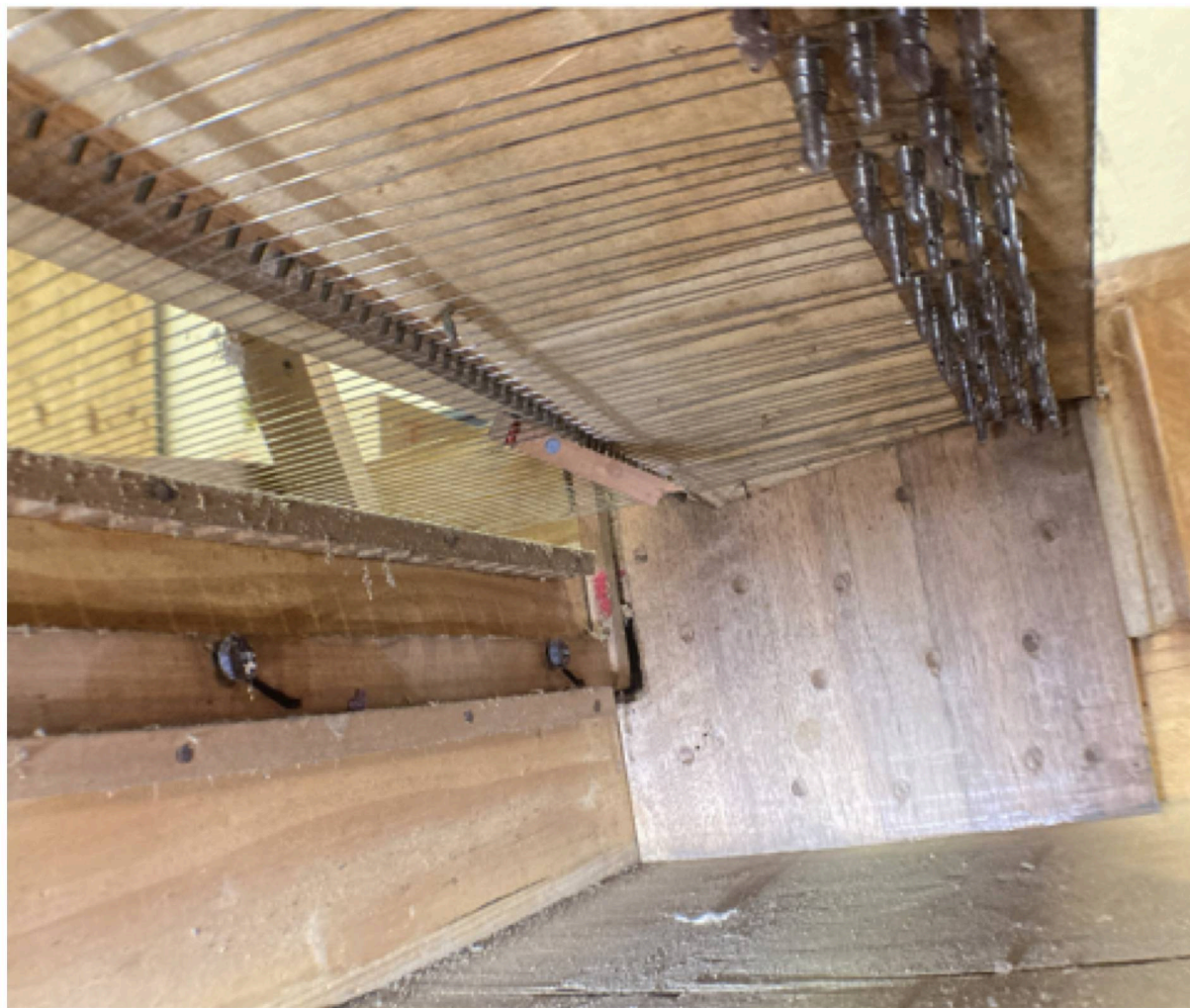
J.K. Mercken wrestplank under view, treble (a broken damper hangs between strings).
