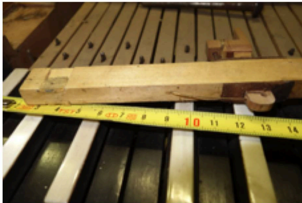
J.K. Mercken c.1768: Key with escapement hopper, intermediate levers (photos CC, KS)
