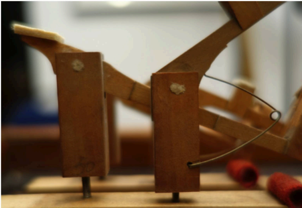
C. Baumann c. 1785 Kapsel pivots of silk floss
